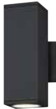
61352 Nottawa Dimmable LED Up and Down Light Wall Fixture with Color Temperature Selection Black Finish Frosted Glass Panels Height: 10.25" Width: 4.50" Extends: 5.75" Height from Center of Outlet Box: 5.04" Back Plate: H: 4.37" W: 4.37" Includes (2) x 9 Watt Integrated LEDs 1,080 lumens, 50,000 hours
