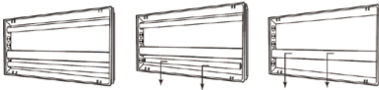
a) Troffer and lamps b) Remove tube lamps c) Remove ballast cover (lens removed)
